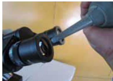
Figure 4 blowing off the dust particles from eye pieces
